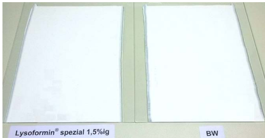
Figure 2: Appearance of the sample by 10 strains with 1,5% - Lysoformin Spezial solution compared to unstressed sample (blank BW)
