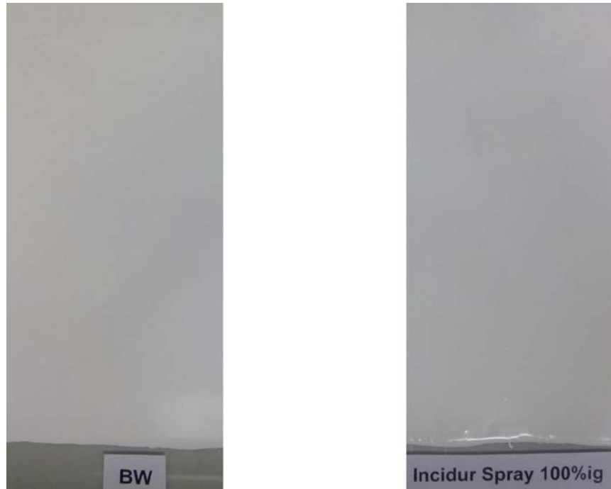
Figure 3: Appearance of the sample by 10 strains with 100% - Incidur solution compared to unstressed sample (blank BW)
