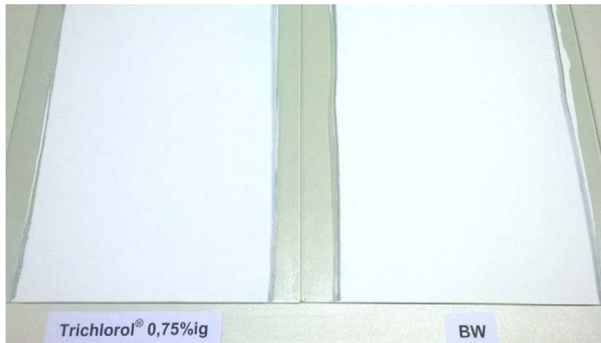
Figure 1: Appearance of the sample by 10 strains with 0.75% - Trichlorol solution compared to unstressed sample (blank BW)
